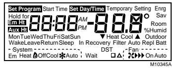
Fig. 8. LCD segments display.
