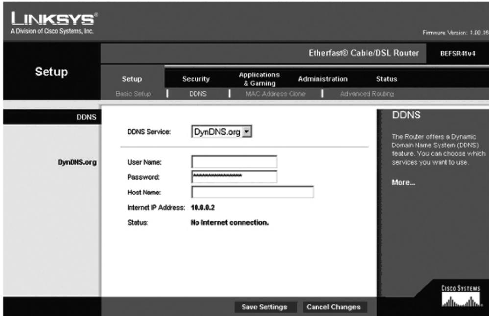
Fig. 8. DDNS setup screen.
