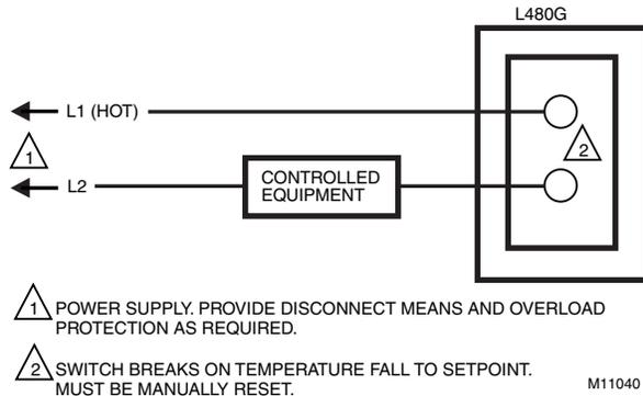
**Fig. 4. Typical hookup for L480G Temperature Controller.**
