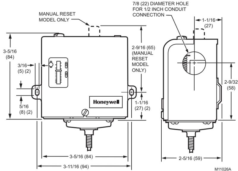
Fig. 1. L480 Temperature Controller dimensions in in. (mm).
