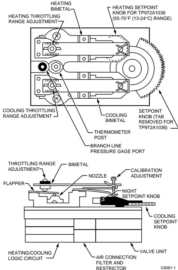
**Fig. 16. TP972A and TP9620A Cross Section Showing Adjustments and Modular Construction.**
