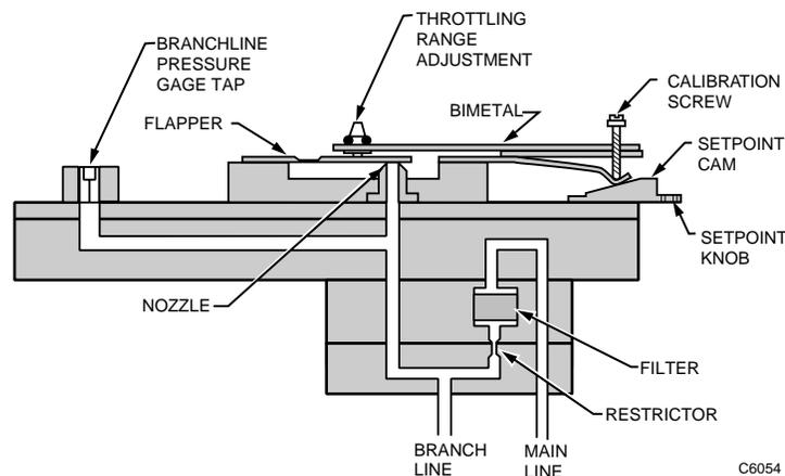
**Fig. 9. Cross Section of TP973 and TP9630 Thermostat.**
