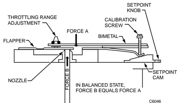
**Fig. 1. Flapper-Nozzle-Bimetal Assembly.**
