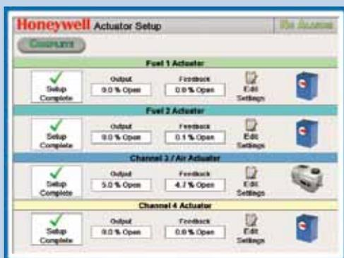
The actuator setup routine steps through the process and shows the status of each
