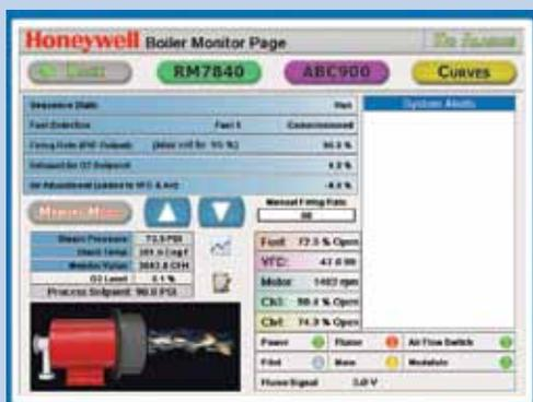
Easily monitor the status of the boiler and controls on the monitor page either at the panel or remotely by tying it into your BAS
