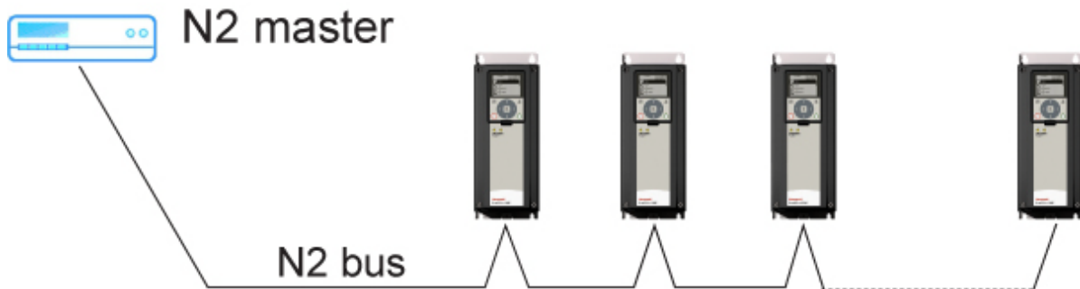
Figure 4. Principal example diagram of Metasys N2
